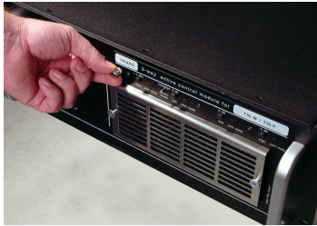
1) Unscrew silver knob on the controller-module
